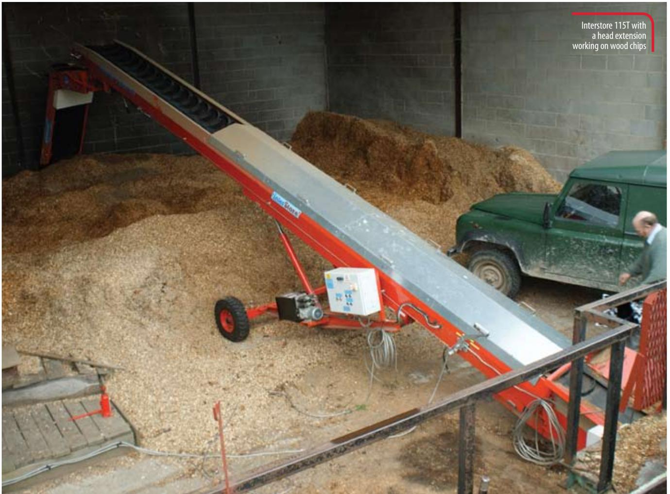
Interstore 115T with a head extension working on wood chips
